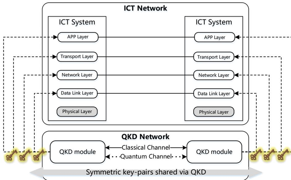
**Figure 9-1: QKDN integrated with TCP/IP protocol stack**
