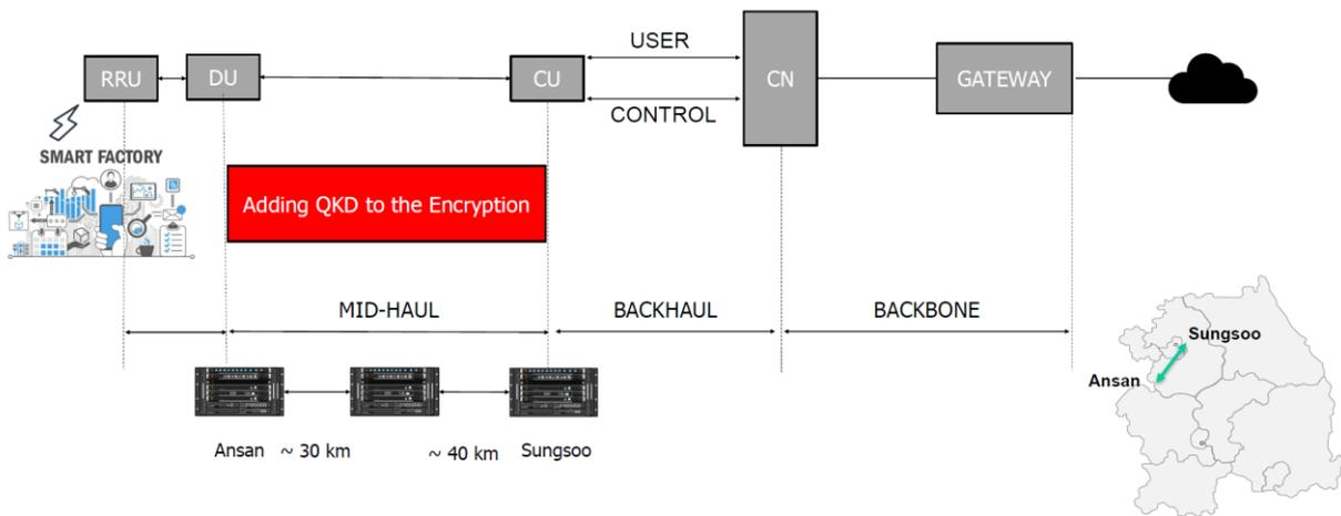
**Figure 12-5: 5G mid-haul QKD deployment for smart factory**
