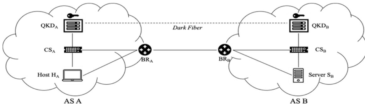
**Figure 12-17: High-level overview of the SCION-QKD integration model**
