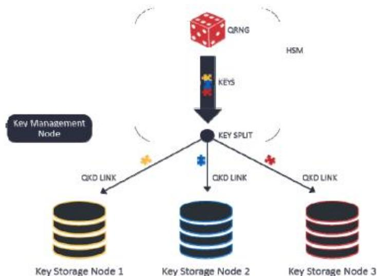
Figure 12-16: QKD in a quantum-secured blockchain vault
