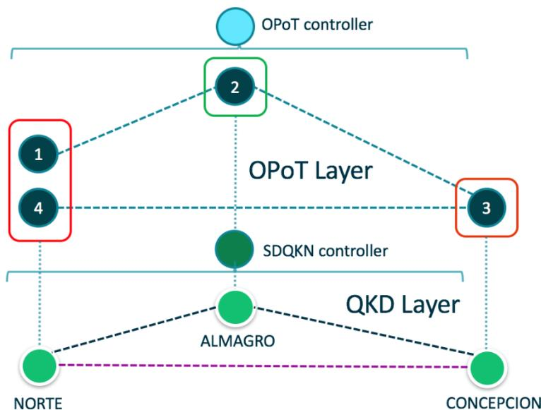
**Figure 12-15: OPoT-DEM: setup for the ordered proof of transit to secure service chaining as was used in the Madrid quantum network**
