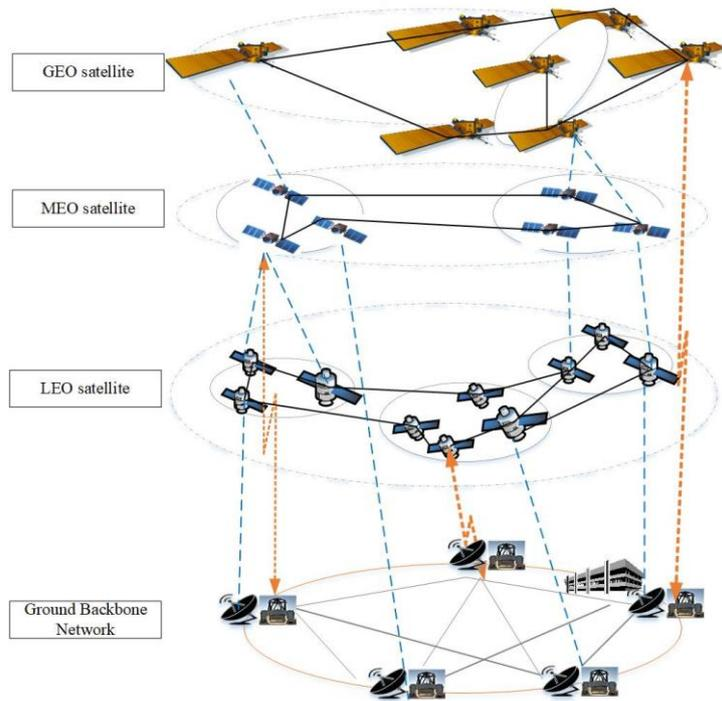
**Figure 10-2: Architecture of general-purpose long-haul network based on multi-layer satellites**
