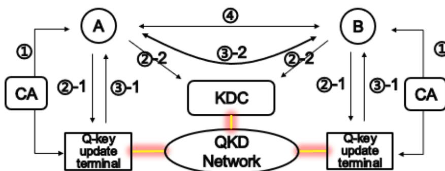
**Figure 11-4: QKD-key embedded secure mobile communication solution**
