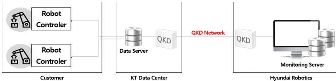
**Figure 13-1: QKDN for smart factory**
